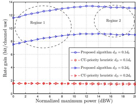
Fig. 8. The rate gain with  $N = 4$  for  $d_D/d_0 = 0.1, 0.2$ .
