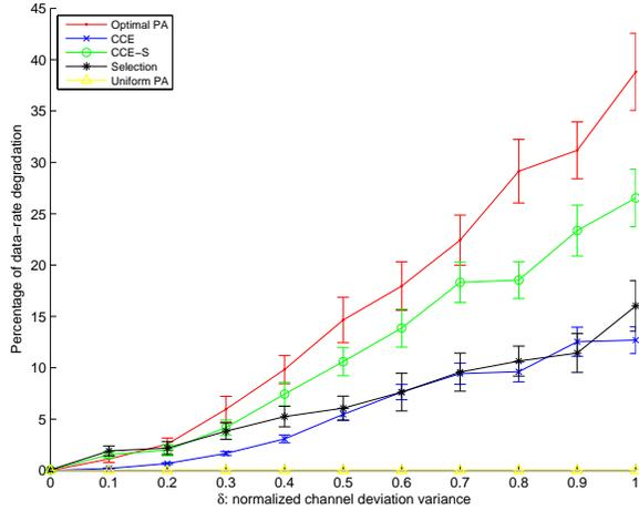
Fig. 5. Percentage of data-rate degradation vs. normalized channel deviation variance for source-centered relay placement
