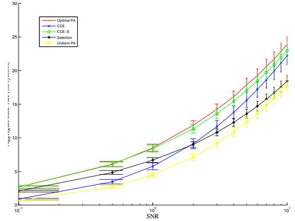
Fig. 1. Aggregate data-rate (bit/symbol) vs. SNR for distributed relay placement
