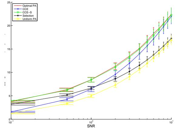
Fig. 3. Aggregate data-rate (bit/symbol) vs. SNR for destination-centered relay placement
