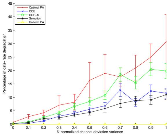
Fig. 6. Percentage of data-rate degradation vs. normalized channel deviation variance for destination-centered relay placement
