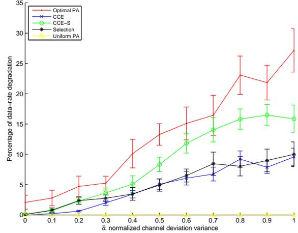
Fig. 4. Percentage of data-rate degradation vs. normalized channel deviation variance for distributed relay placement
