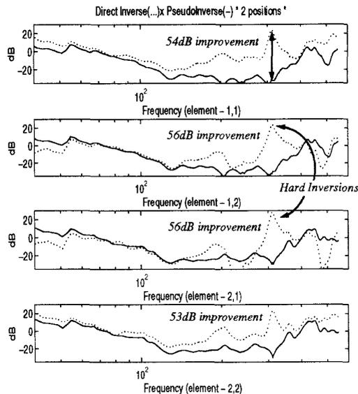
Figure 5 shows the results of the equalization, which plots the spectrum of frequencies for each microphone position, before (dotted line) and after (solid line) the desired vector and the new “pseudo” inverse have been found and applied for equalization.
